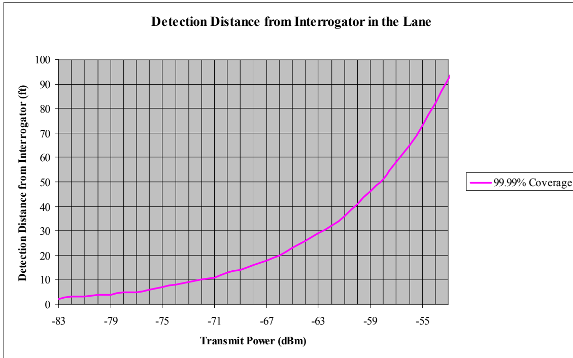
Figure 23: Detection Distance vs Transmit Power for Stored Container Scenario
